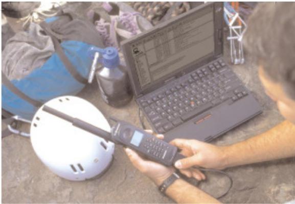
Fig. 2: Satellite systems may be interfaced with computers for asset tracking or other mapping applications.
