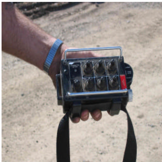
Fig. 3: Remote control apparatus uses attached controls. This configuration also allows him to stand further away from the machine and see more of the movement.
