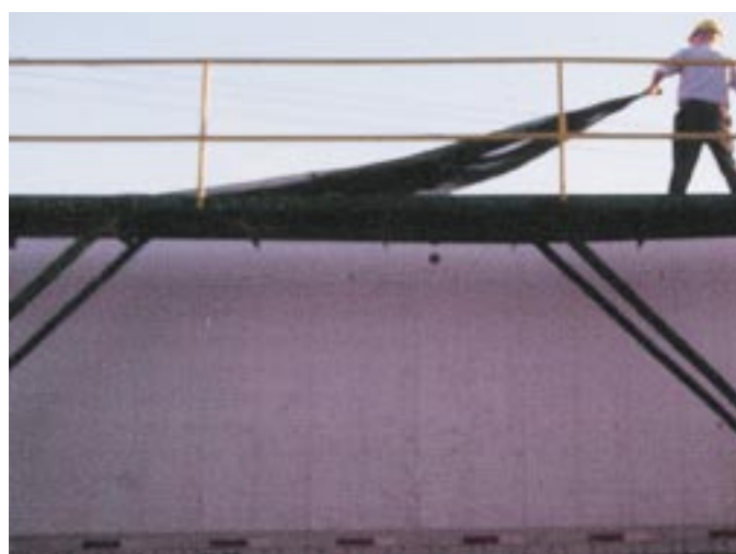
Fig. 6: Driver pulls/rolls tarp from safety of the catwalk.
