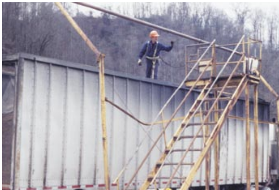
Fig. 4: This Virginia sawmill/chip mill's tarping station includes a safety harness and chain tether for the truck driver . . .
