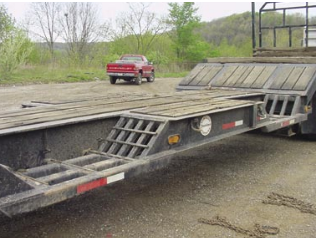
Fig. 1: Wheel wells are built into the multi-purpose trailer.
