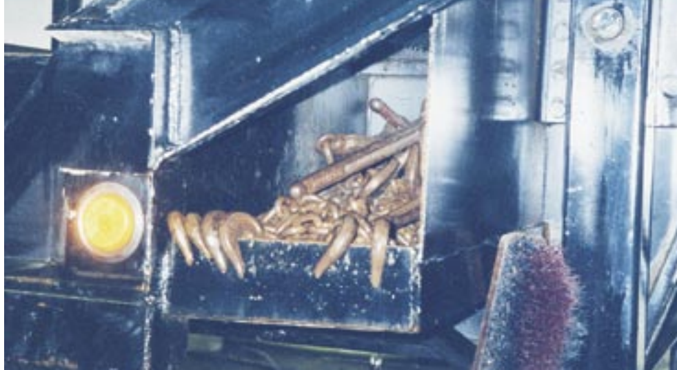
Fig. 3: Metal compartment for chains and binders is built on each side just behind the landing gear.
