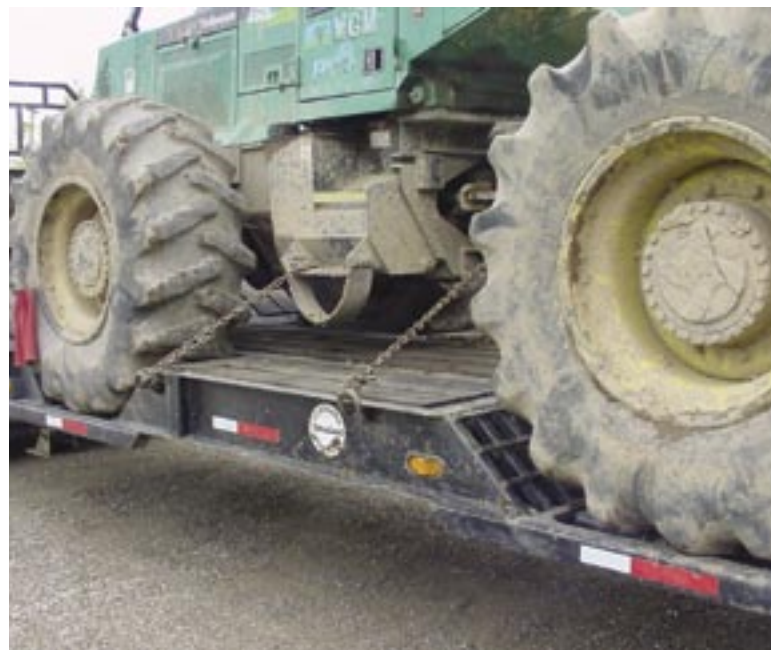
Fig. 2: Skidder sits safely and securely in wheel wells during transport.
